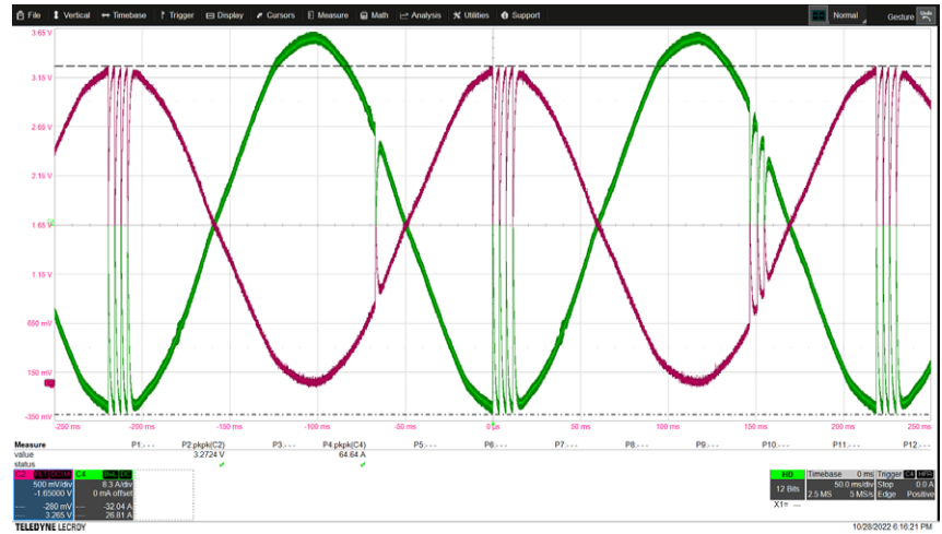
Figure 4. Phase current and current sense signals. Note that the voltage threshold is positive, but the kelvin connections on the shunt resistor make the overcurrent circuit active at negative current values. As measured by the cursors, the overcurrent threshold is set at -32 A
